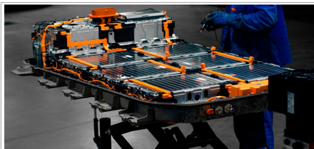
[Figure 4-5] Battery Inspection and Insulation Measurement
