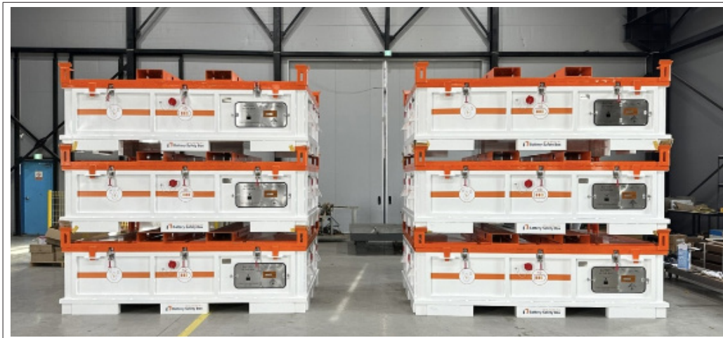
[Figure 4-4] Explosion-proof Equipment for the Safe Transportation of Used Batteries
